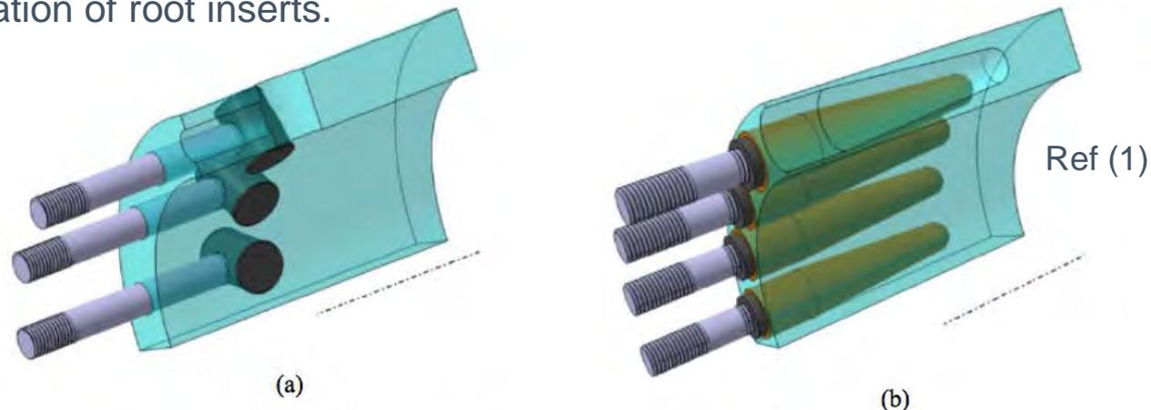
**Figure 1. Common root connectors (a) T-Bolts (b) Bonded inserts**
